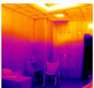
Poor circulation of air is shown in this room. Notice the warm air at the top of the room and the cool floors, blue. Commonly referred to as the "Stack Effect".
