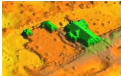
2004 lidar, 0.5m resolution DEM binned and computed by RST (smoothes out the noise and fills in the gaps)
