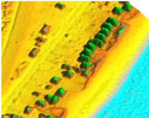
1m res. DEM, computed by RST, 1998 lidar data
