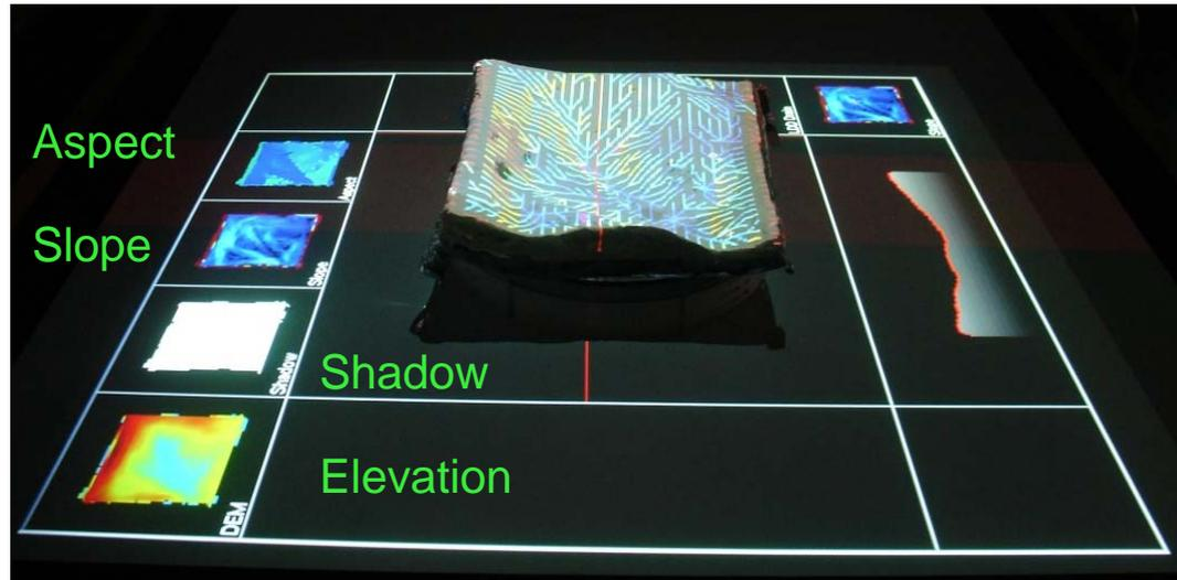
Model is continuously scanned while flow direction, slope, elevation change, profiles are computed in real time and projected over the model or workspace.
