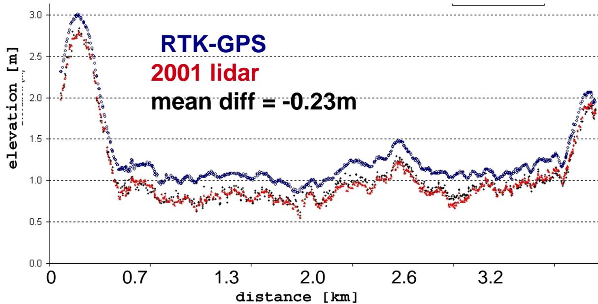
Elevation difference between RTK-GPS survey (0.03m RMSE) and lidar data along centerline of a stable road (NC12).
